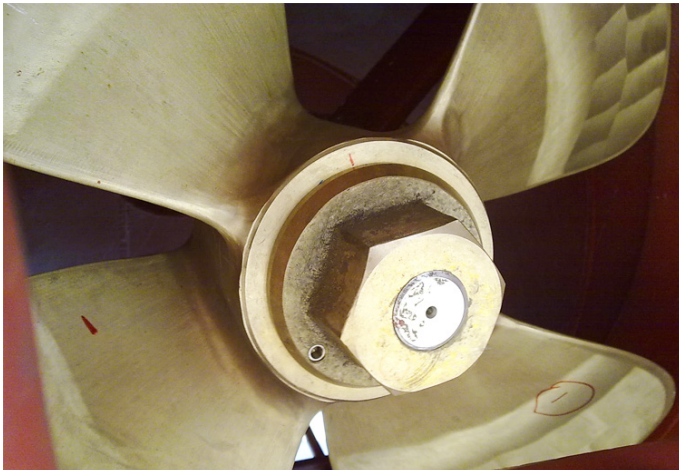
Fixed pitch propeller, optimized for the thruster dimension and motor power.
