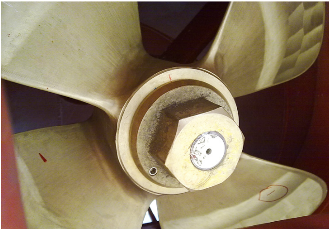
Fixed pitch propeller, optimized of the thruster dimension and motor power.
