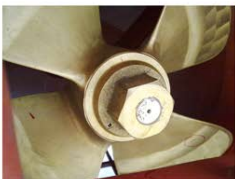
Fixed pitch propeller, optimized of the thruster dimension and motor power.
