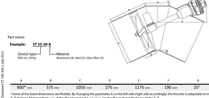
\*Some of the listed dimensions are flexible. By changing the parameter A on the left side (right side accordingly) the thruster is adaptable to most hull designs. Material thickness of the thruster tunnel is equal or greater the material thickness of the hull
