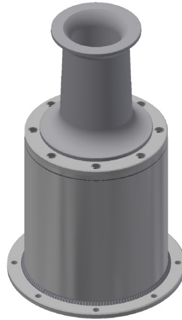
C3000D L400: Custom deck mounted 3 000kg capstan
