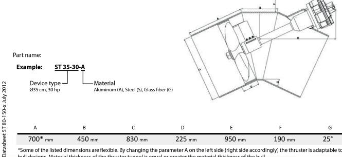
\*Some of the listed dimensions are flexible. By changing the parameter A on the left side (right side accordingly) the thruster is adaptable to most hull designs. Material thickness of the thruster tunnel is equal or greater the material thickness of the hull
