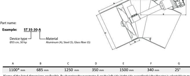
\*Some of the listed dimensions are flexible. By changing the parameter A on the left side (right side accordingly) the thruster is adaptable to most hull designs. Material thickness of the thruster tunnel is equal or greater the material thickness of the hull
